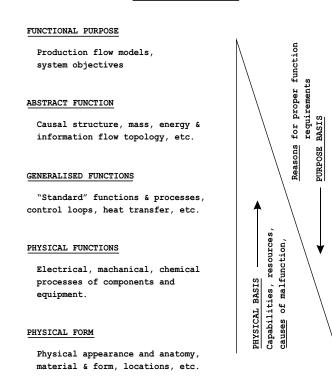
Fig. 3. Properties of system will be used in operators' decisionmaking in terras of concepts at several levels of abstraction; frequently even during single decision sequence.
